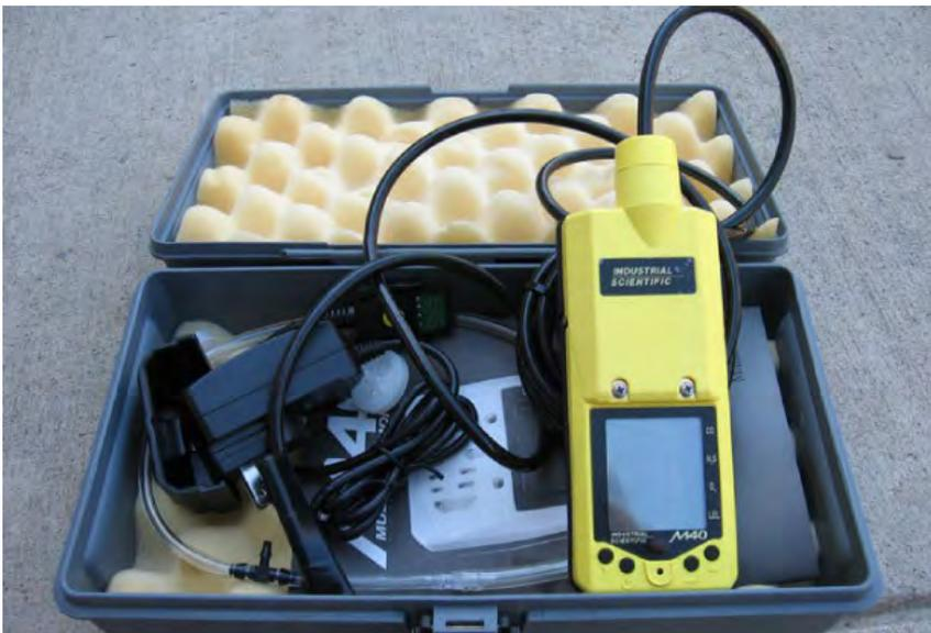
Figure 1. An example of a handheld, portable gas monitor with probe and hose.
