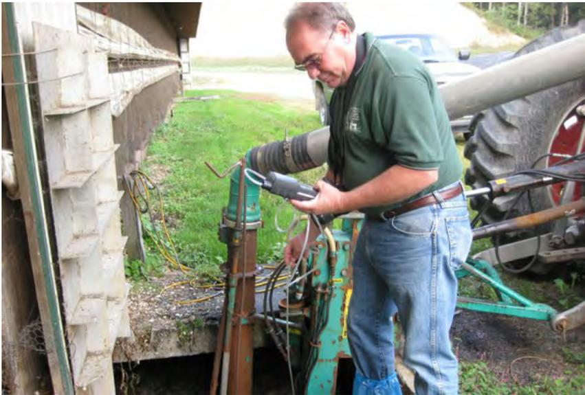
There are many manufacturers of portable gas monitors in a price range from \$250 to over \$1,400. Many are programmed for monitoring manure gases and to detect oxygen depletion. Purchasers or leasees should ensure that the multi-gas detectors they are considering have the capability for detecting hydrogen sulfide and methane, and also oxygen deficient environments within the 0-30% by volume range.
