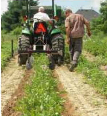
Eric Vanderhyde testing hilling disks on his new SARE funded easy change-out tool bar.
