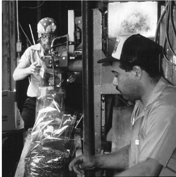
Figure 4. Filling nutrient supplemented sawdust substrate into heat-resistant polypropylene bags for heat treatment.
