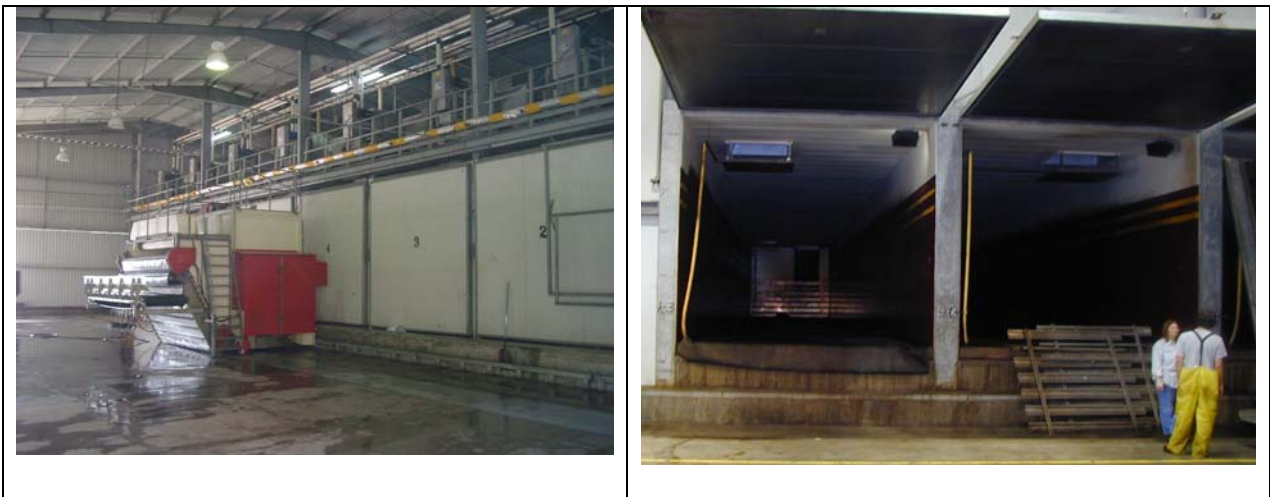
Figure 2. Phase II tunnels used to pasteurize and condition compost for mushroom production. Left: filling machine in front of closed tunnel, Right: open tunnel ready for filling.
