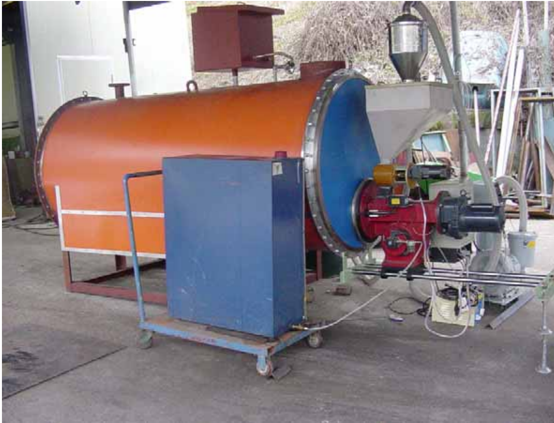
Figure 3. Shown is the GR Technologies boiler at the factory in Korea. The rectangular tank in the foreground stores the fuel oil for pre-heating. The boiler is the cylindrical piece on the left behind the fuel tank. The high-temperature burner is shown on the right, fueled by plastic pellets conveyed by a vacuum feed device to the hopper atop the burner. The electronic control box is partially visible behind the burner.
