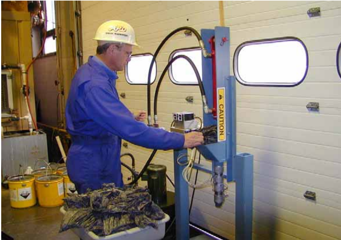
Figure 1. Shown are very dirty plastic drip irrigation tubing and mulch film being fed by hand into the prototype Plastofuel machine. A hydraulic cylinder forces the plastic items through a heated die, shown on the lower right. The extruded material is then cut with a hot knife to form Plastofuel, shown in Figure 2.
