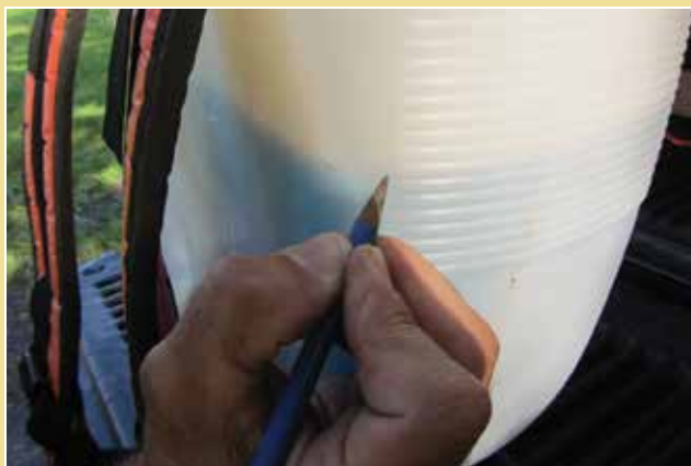
When using the subtraction method, mark the starting water level in your sprayer, treat the calibration area, and determine by subtraction the volume sprayed as you refill the sprayer to the starting point. Photo: Kimberly Bohn
