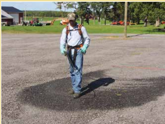
Time how long it takes to treat the calibration area, 340 square feet. Operate the backpack as you would when spraying in the field, getting uniform coverage while walking at a comfortable speed. (Note: This level of wetting is heavier than operational to enhance the pattern for the purposes of this image.) Photo: Kimberly Bohn
