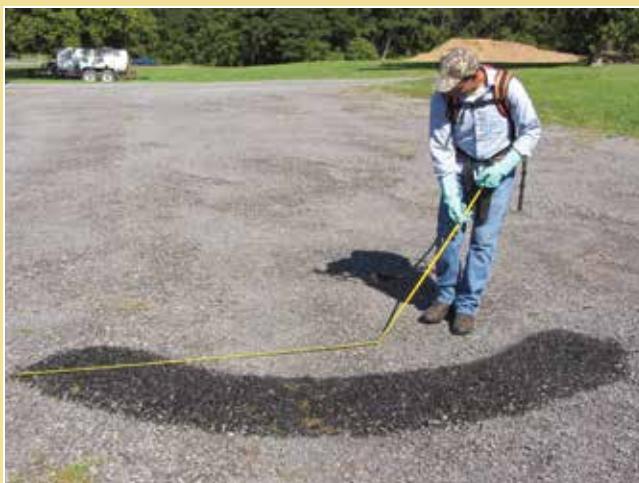
Using an adjustable cone nozzle and moving the spray wand back and forth slowly will increase the band width, thus providing greater coverage. Here our band width is 9 feet. Photo: Kimberly Bohn
