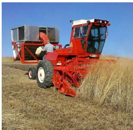
The self propelled harvester, with a body width of 8 ft, drives only in the path where the biomass was removed. This feature of the harvester reduces the land area needed for a research project by enabling different research treatments to be grown adjacent to each other and harvested individually. Reducing the land area reduces the variability in the research and maximizes the ability to detect treatment differences.
