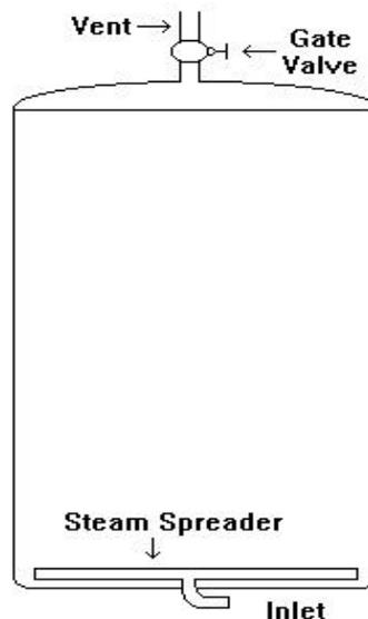
Specifications. A 1-inch vent in lid or top side, equipped with a 1-inch gate or plug cock valve and discharging directly into the atmosphere or to a manifold header.
