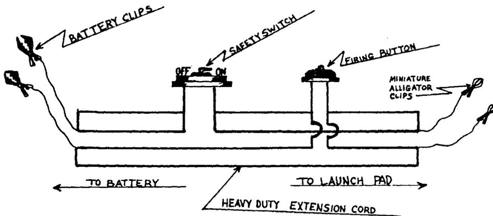
Figure 2. Schematic Drawing of Wiring for Launch Panel
