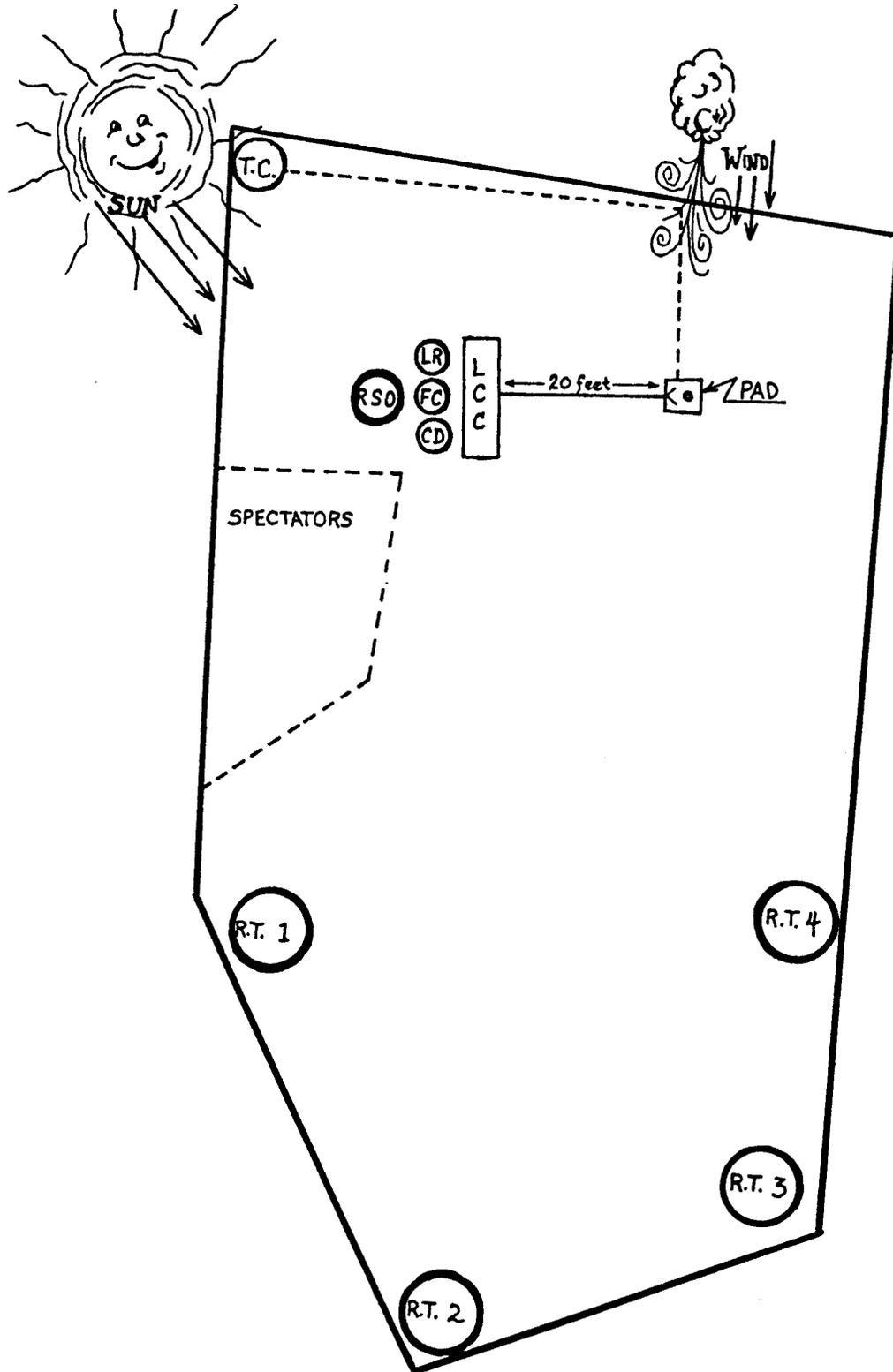
Figure 7. Model Rocket Launch Range
